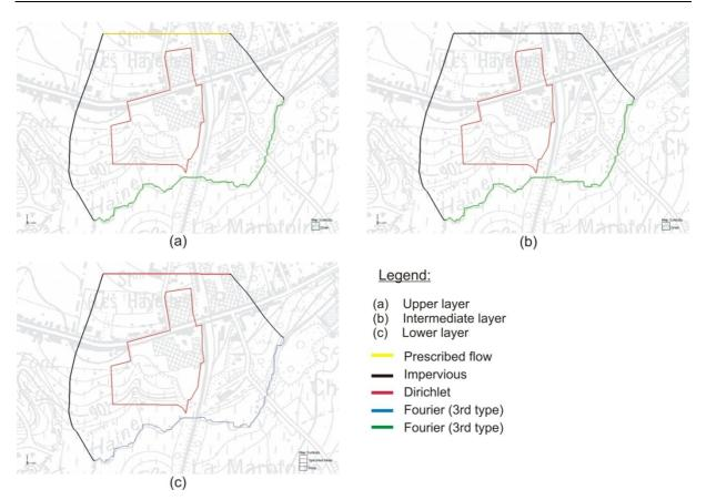
Figure 6: Boundary conditions considered at the various limits of the finite difference model. At the top of the model, a Neumann (prescribed flux) is also applied to account for pluviometric recharge.
