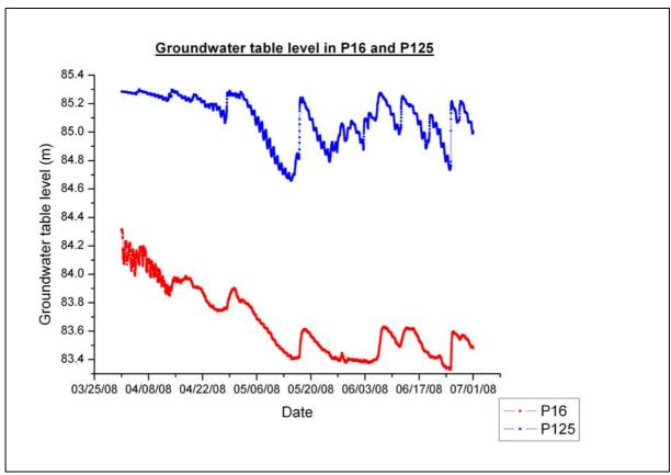
Figure 21: Groundwater table levels in the upper aquifer (P125) and in the lower aquifer (P16)
