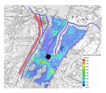
Figure 4: Advective transport of pollutants simulated with MODPATH coming from the SRI/BIOLUX-site (colors are providing groundwater fluxes in m3/day)
