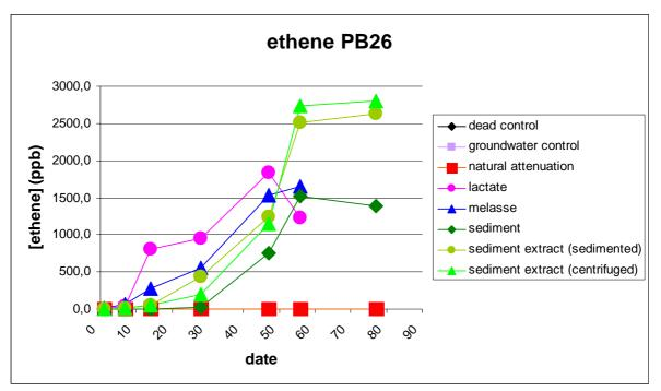
Figure 10: (Stimulated) degradation of DCE and subsequently VC to ethene at the location Pb 26 at the Vilvoorde-Machelen site.
