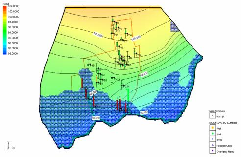
Figure 7: Calculated hydraulic head contours for the upper aquifer layer.
